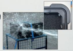
EXOcase lids have standard neoprene joints and provide IP 56 protection.
